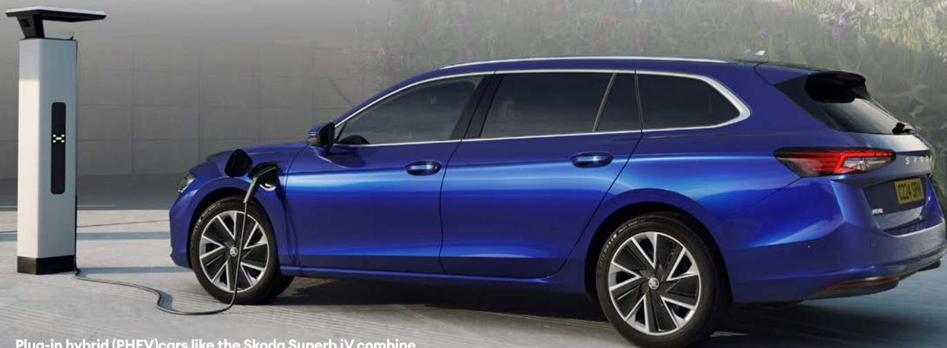
Plug-in hybrid (PHEV) cars like the Skoda Superb iV combine battery electric power and a traditional combustion engine and are a good option for those who aren't ready to go fully electric
