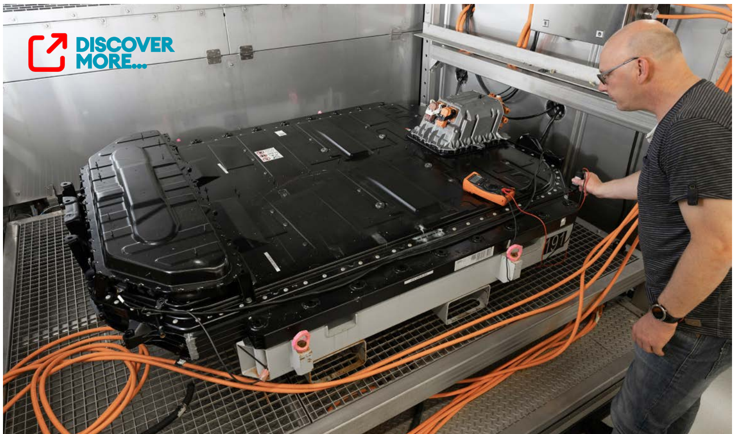
Audi invited us to see its battery testing facility in Germany where technicians can simulate a complete lifetime of use and abuse. Only when packs survive the equivalent of 15 years of charging and driving are the designs approved for production
